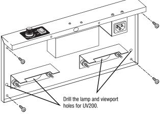
**Fig. 5** Mount the device using included sheet metal screws.
