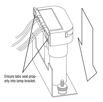
**Fig. 8** Insert the lamp fully, making sure the electrical connector seats properly into the lamp bracket.
