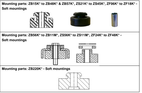
Figure 2: Mounting parts
