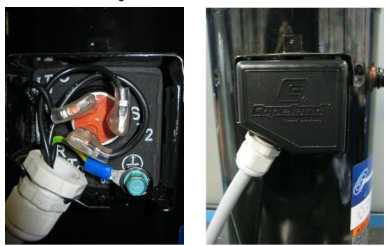
Figure 14: Correct electrical installation with cable glands for IP21 T-box (models ZB15K\* to ZB45K\*)
