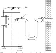
Figure 10: Suction tube design
