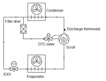
Figure 4: Liquid injection with DTC valve
