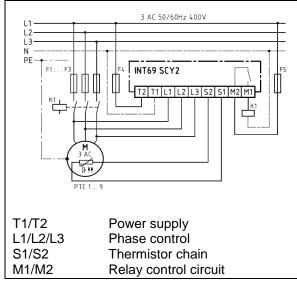
Figure 18: Wiring of the motor protection module
