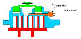
Figure 17: Internal discharge temperature sensor position
