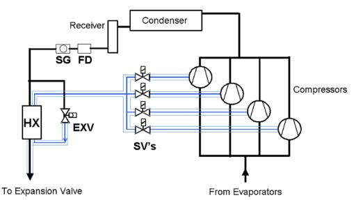
Figure 8: Vapour injection line diagram
