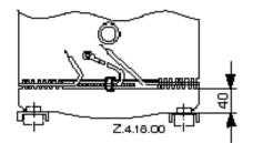
The crankcase heater must be mounted tight to the shell 40 mm above foot plate (see **Figure 12**).
