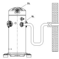
Figure 7: Suction tube design
