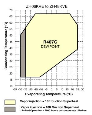
Figure 2: R407C application envelope for vapour injection compressors ZH06KVE to ZH48KVE operating with vapour injection
