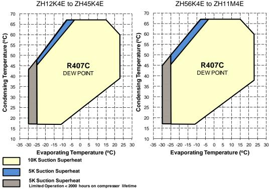
Figure 1: R407C application envelopes for standard compressors ZH12K4E to ZH11M4E
