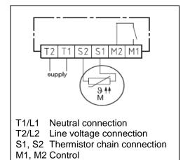
Figure14: Wiring of the motor protection module
