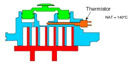
Figure 13: Internal discharge gas temperature sensor position for models ZH56K4E to ZH11M4E and ZH24KVE to ZH48KVE
