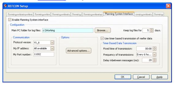
To have the Planning System Communication Interface work, first of all make sure the "Enable" checkbox is checked. Also decide the configuration as described in the following.
