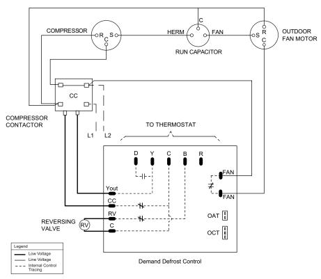
Fig 1. Typical System Wiring Diagram
