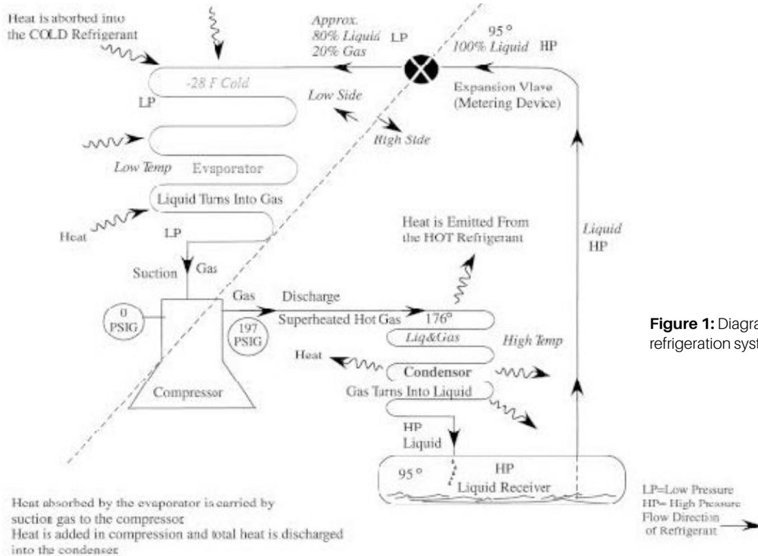
Figure 1: Diagram of a typical refrigeration system
