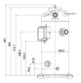
Figure 2: Dimensions ZBD30K\* to ZBD57K\* & ZFD13KVE to ZFD25KVE
