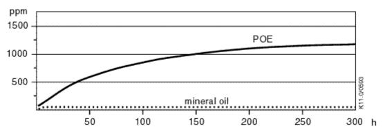
Figure 23: Absorption of moisture in ester oil in comparison to mineral oil in ppm by weight at 25°C and 50% relative humidity (h=hours)
