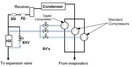
Figure 12: Vapour injection line diagram
