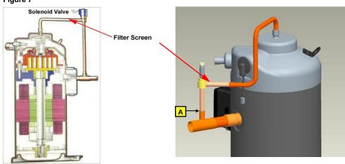
Figure 8: Position of external solenoid valve Figure 9: Recommended piping
