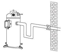
Figure 16: Suction tube design
