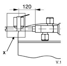
The R404A, R407A, R407F, R448A and R449A dedicated discharge thermostat has a cut-out setting of  $130^{\circ}C \pm 4K$  with closing at  $101^{\circ}C \pm 8K$ . The thermostat should be installed approximately 120 mm from the discharge valve outlet (see **Figure 22**). It must be insulated in order to avoid improper functioning due to false readings (see "X" in **Figure 22**).
