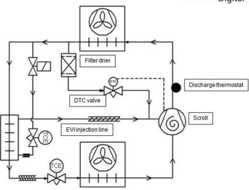
Figure 13: Wet vapour injection cycle for R407A & R407F low temperature applications
