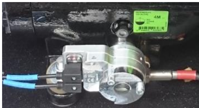
Figure 47: OW5 TraxOil mounted on the compressor
