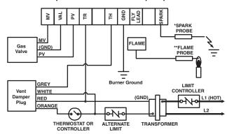
Fig. 4 – Typical hookup for White-Rodgers replacement with vent damper and separate flame-sense and spark probes
