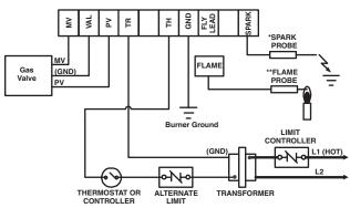
Fig. 2 – Typical hookup for White-Rodgers replacement with separate flame-sense and spark probes
