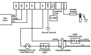
Fig. 3 – Typical hookup for White-Rodgers replacement with direct flame sense throughsingle spark/sense probe
